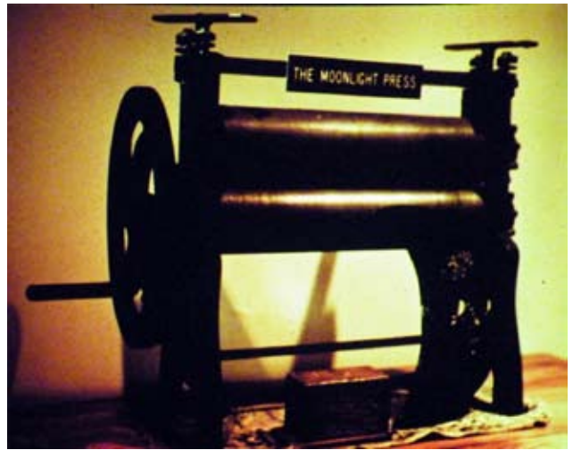
Antique Sheet Press (Mangler) turned Printing Press "The Moonlight Press" adapted by Chris Spollen - early 1970s Cast Iron and Steel
